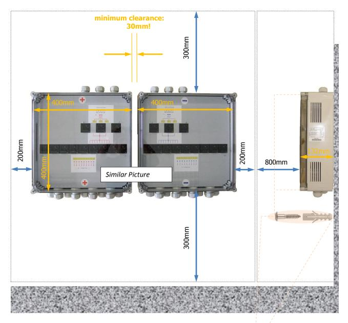
Select the correct mode of mounting, <u>depending on the mounting</u> <u>surface</u>, for example 4 x expansion anchor "S8"+ 4 x chipboard screw Ø5.0
